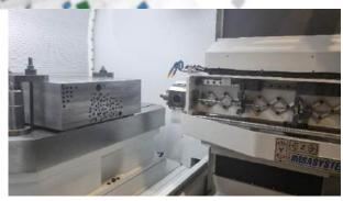
MF 1200 D is a CNC machine with 4/5 axes for deep drilling by gun drill tool, in molds and blocks up to 4 tons. Swing clearance 1.250 mm, table load 4.000 kg. MF 1200 D can be equipped with standard fixed table (4 CNC axes) or optional rotary table (5 CNC axes).
