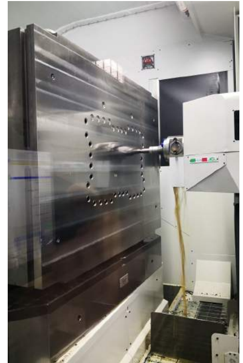
The 500th I.M.S.A. drilling machine in operation at Exacta Stampi in Brianza, Italy (model MF1350EVO).
