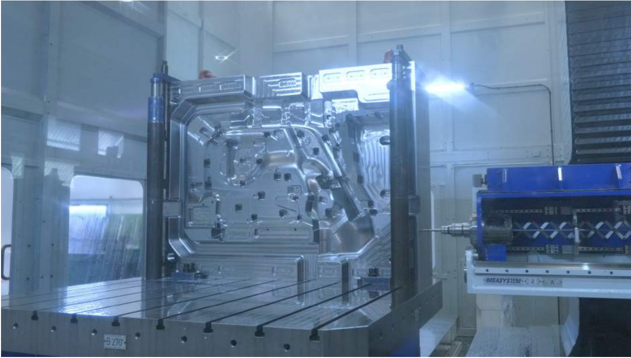
Deep drilling and milling machine with MF1600S angled machining unit for the machining of molds up to 20 tons
