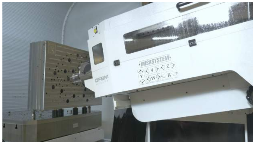
The MF1450BB model, the new BB-Evo series, is designed for molds up to 12 tons.
